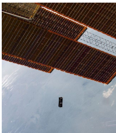
Nanosatellite being launched from ISS (Courtesy of JAXA/NASA)
